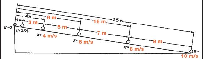
a. Do you see that the total distance from the starting point increases as the square of the time? This was discovered by Galileo. If the incline were to continue, predict the ball's distance from the starting point for the next 3 seconds.
