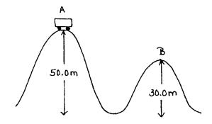
**Solution:** Because mass is contained in each of these equations, it cancels out and does not need to be included in the calculation. Also, the inclination of the hill makes no difference. All that matters is the change in height.
