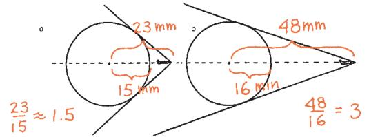
Aircraft (a) is traveling about <u>1.5</u> times the speed of sound.
